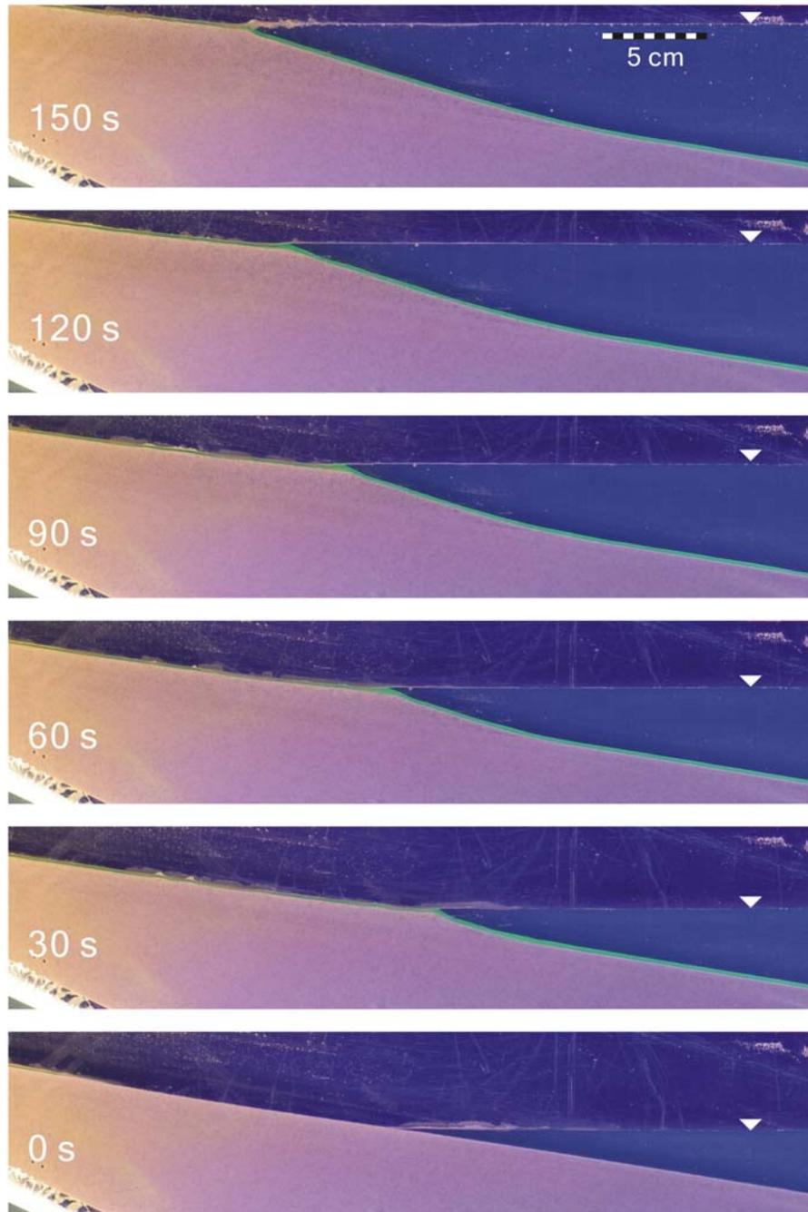
Figure 5. Series of experimental photographs depicting the progradation and subsequent retreat of a hyperpycnal delta subject to a steady rise in base level.
