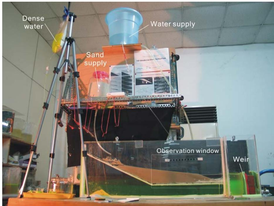
Figure 4. Experimental set-up used for the small-scale laboratory experiments.
